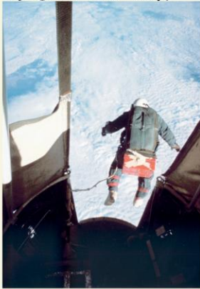
FIGURE 1 Stratospheric leap into history. Moments into Captain Joseph Kittinger's historic exploration of the atmosphere, captured by a remotely triggered camera. The lanyard cord is attached to his parachute pack and snaps to set a timer that opens a small stabilization chute 16 seconds into the free fall. The clouds are more than 26,000 m (85,000 ft) below him. He carries an instrument pack on his seat, his main chute, and pure oxygen for his breathing mask. [Volkmar Wentzel/NGS Image Collection, used by permission from the National Geographic Society, National Geographic Magazine , Dec. 1960, p. 855. All rights reserved.]
