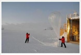
Staff at the South Pole get ready to release a balloon that will carry an ozone instrument up to 20 miles in the atmosphere, measuring ozone levels all along the way. NOAA image from 2011.
