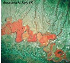
Infrared aerial photography: Developed in WW2 to detect painted targets camouflaged to look like vegetation
