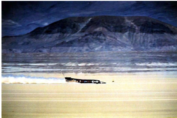
"Thrust SSC" exceeds the speed of sound. Note Mach lines streaming from surface of vehicle.
