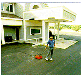
Detection of underground storage tanks (UST's) is a common application.
