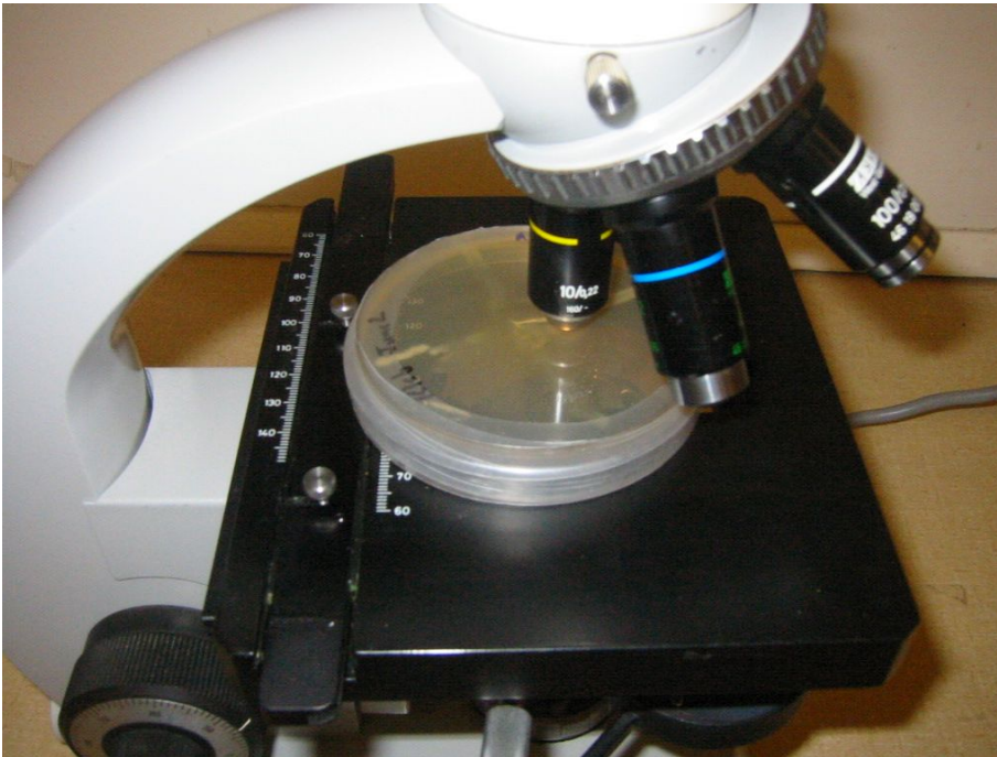
Figure 38 Observing organisms in situ on the surface of an agar plate using a compound microscope.
