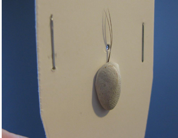
Figure 18 Press the putty with subject attached to the cardstock (thin) side of the microscope with the subject lying over the lens.
