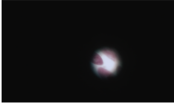
Figure 62 View showing the view through the microscope with the condenser diaphragm completely closed. Note that the majority of the field of view will be dark. The small circle of light indicates the edges of the illuminator diaphragm.
