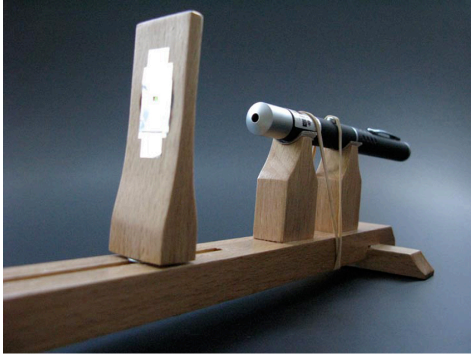
Figure 23 The basic set up for a stand to measure the power of a lens using a laser.
