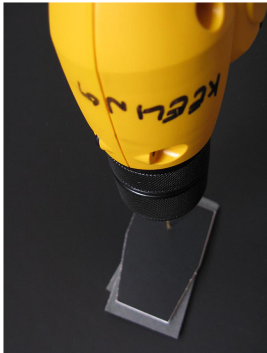
Figure 10 Drilling a hole to hold the lens and create a light path.
