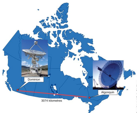
Figure 4.7b The first successful long-distance interferometry experiment was conducted in 1967 in Canada, with the 25.6 m Dominion Radio Astrophysical Observatory telescope in Penticton, British Columbia (left), in conjunction with the 46 m telescope at the Algonquin Radio Observatory at Traverse Lake in Ontario (right) to simulate the resolution of a giant radio telescope measuring 3074 km, the physical distance between the two instruments.
