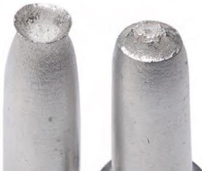
Cup-and-cone fracture in aluminum [1]
