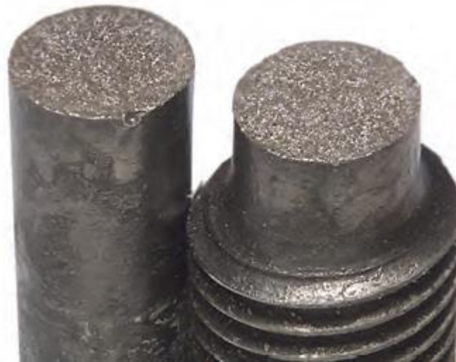
Figure 8: Brittle fracture in a mild steel [1]
