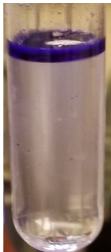
Figure 1.5. 5 ml H 2 O, 0.5 ml 1-butanol, 1 drop 0.003 M aqueous crystal violet after shaking for 10 seconds
