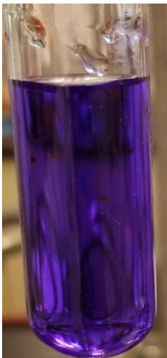
Figure 1.5. 5 ml H 2 O, 0.5 ml 1-butanol, 1 drop 0.003 M aqueous crystal violet after shaking for 10 seconds
