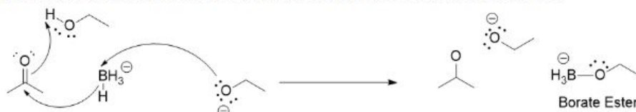
Figure 4.1. Reaction of Borohydride and Carbonyl and the formation of Borate Ester
