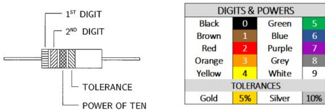
Figure 1. A colour code (Right) displaying the value each colour represents, ranging from digits to powers and tolerance. A diagram of a resistor (Left) showing the order in which the colour slots appear and what they signify.
