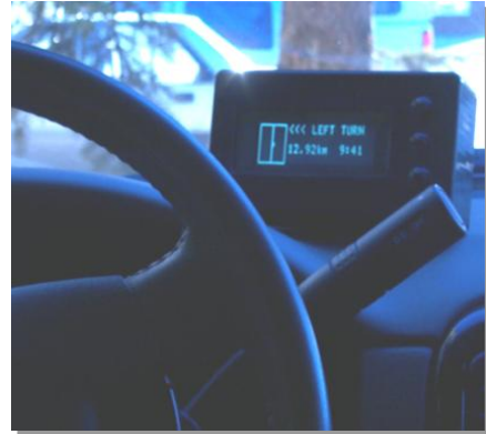
Figure 10.44: Routing Display Installed in an Emergency Services Vehicle
