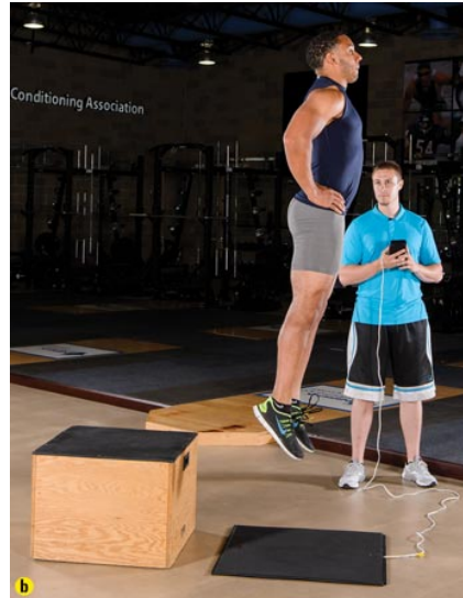
Maximum height: measured by contact mat system Eccentric utilization ratio = VJCM Ht/SVJ Ht
