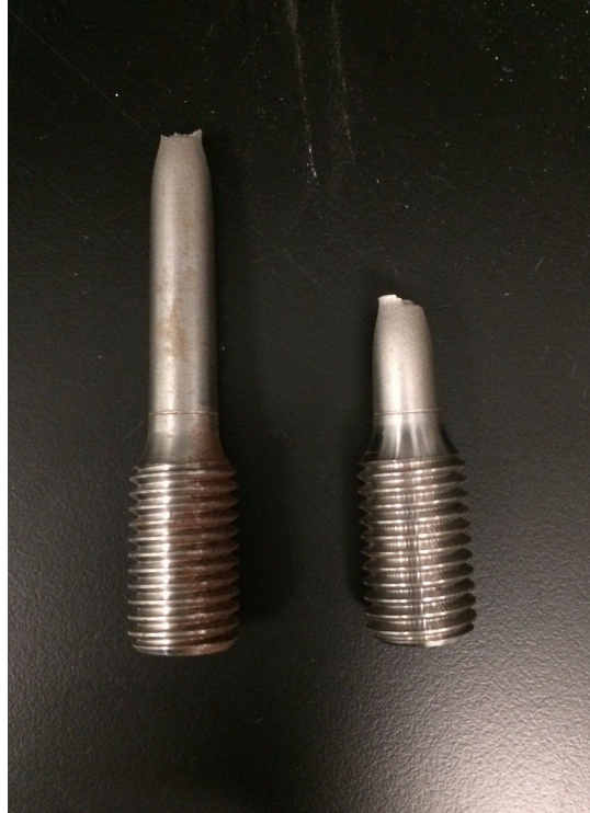
Figure 11: Image of the steel sample after being fractured in the tensile strength machine.
