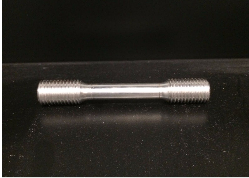
Figure 13: Image of the original aluminium sample before being placed in the tensile strength machine.
