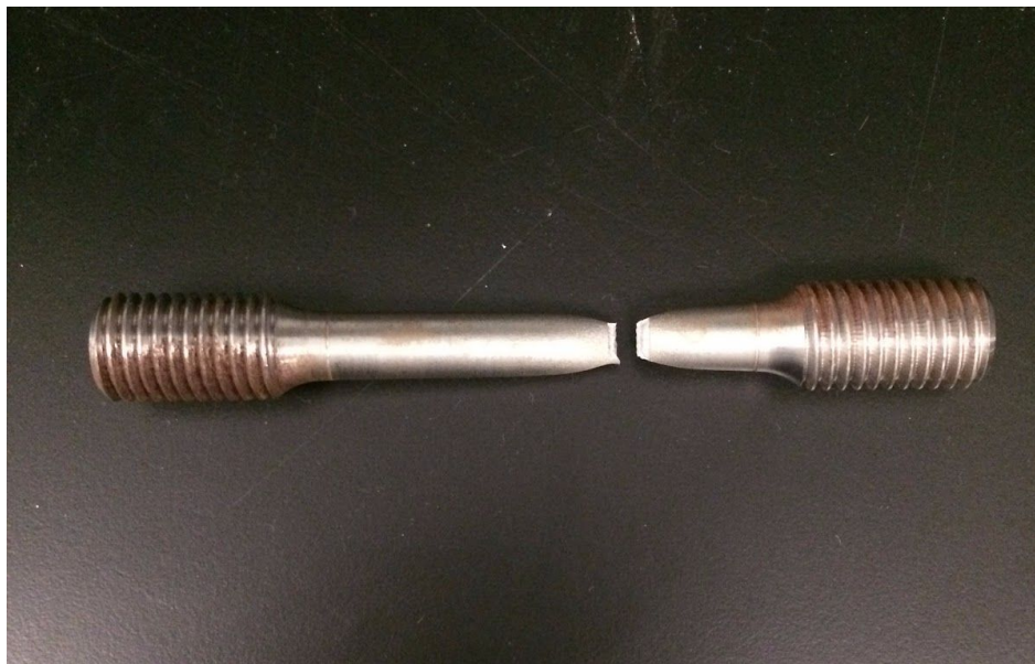
Figure 12: Image showing the steel samples decrease in diameter the closer it gets to the fracture point.
