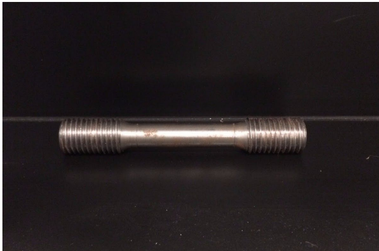
Figure 10: Image of the original steel sample before being placed in the tensile strength machine.
