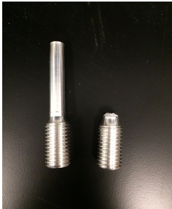
Figure 14: Image of the aluminium sample after being fractured in the tensile strength machine.
