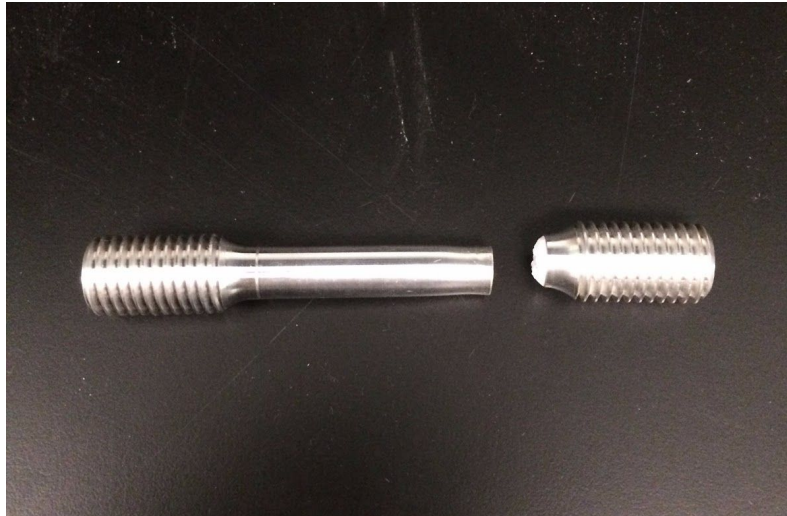
Figure 15: Image showing the aluminium samples decrease in diameter the closer it gets to the fracture point.
