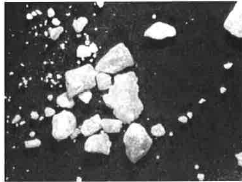
Photo 8: Limestone Debris (x10). White to greyish limestone debris.
