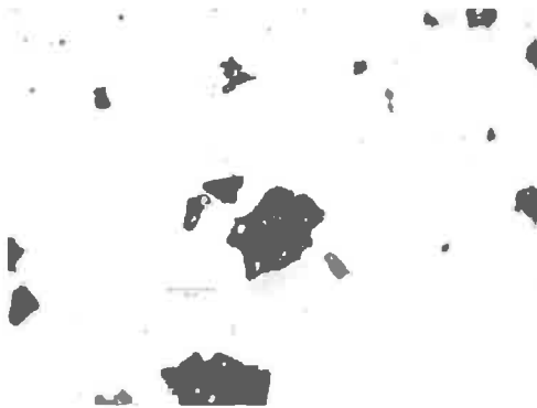
Photo 3: Coke (x25). Opaque, black, sharply angular with rough highly reflective surface.
