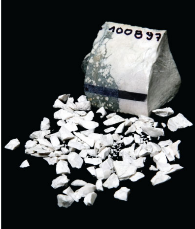
◆ Figure 2.A Core sample of jadarite, a newly discovered mineral with nearly the same chemical composition as the fictional kryptonite—Superman's least favourite substance.
