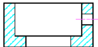
Incorrect cutting plane line
