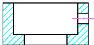
Correct cutting plane line
