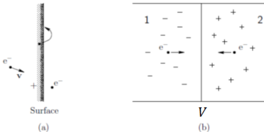
Figure 1:(a) Potential barrier at the surface of a metal. (b) Potential difference due to the electron distribution at the junction between two different metals.
