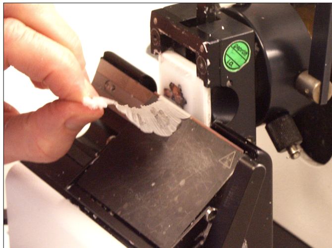
Microtome: cutting thin, paraffin-embedded sections for light microscopy
