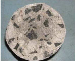
Concrete exposed to CO 2
