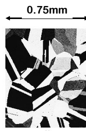
micrograph of Brass (Cu and Zn)
