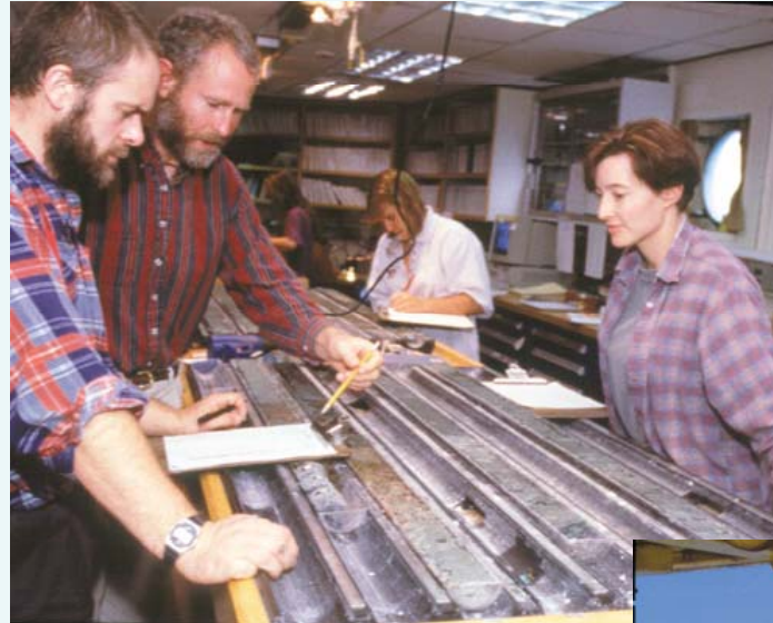
sediment core logging
