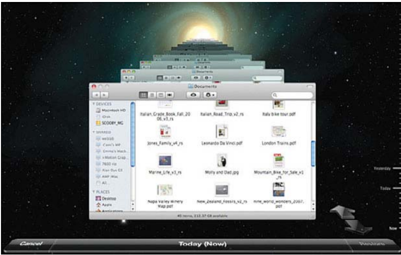
Figure 6.36 Mac's Time Machine restores files, folders, libraries and, if necessary, the entire system.
