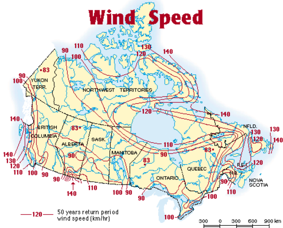
Figure FS.6 A map of Canada showing contours of wind speed (in km per hour) with 50-year Return Periods. Map from Environment Canada.
