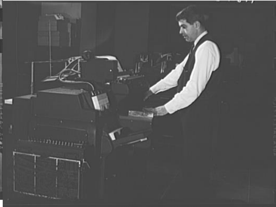
Operator Jack Keefe, in the IBM room of the Office of Defense Transportation feeds the coded punched cards into the tabulating machines (June 1942) (Albert Freeman, Library of Congress)
