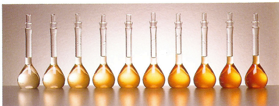
COLOR PLATE 13 Beer's Law (Section 19-2) \text{Fe}(\text{phenanthroline})_3^{2+} standards for spectrophotometric analysis. Volumetric flasks contain \text{Fe}(\text{phenanthroline})_3^{2+} with Fe concentrations ranging from 1 mg/L (left) to 10 mg/L (right). The absorbance, as evidenced by the intensity of the color, is proportional to the iron concentration.
