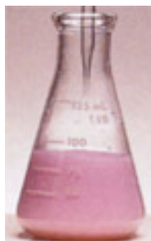
indicator adsorbed on precipitate after endpoint
