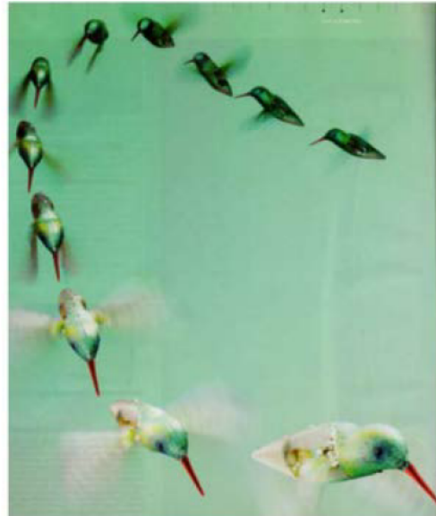
AeroVironment Hummingbird displaying its maneuverability: b = 19 \text{ cm} , W_{\text{total}} = 19 \text{ g} , V = 11 \text{ mph} , Duration \sim 11 minutes.
