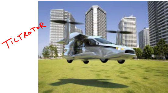
In takeoff or landing mode, the TF-X is a stop/fold tiltrotor with two 600-hp electric motors in nacelles at the tips of the wings.
