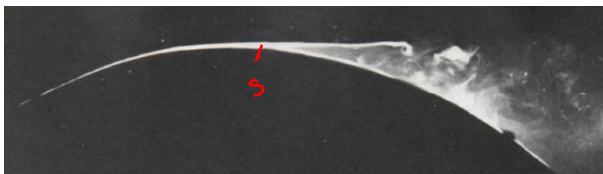
Viscous flow; turbulent boundary layer
