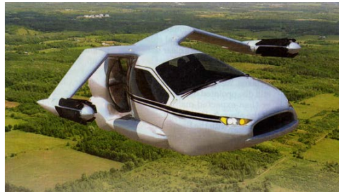
In flight mode, the TF-X uses a 300-hp ducted fan for thrust, giving a non-stop range of 500 mi.
