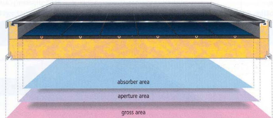
cross-section of a flat-plate collector
