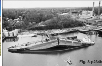
Fatigue Fracture – Cyclic loading from Waves
